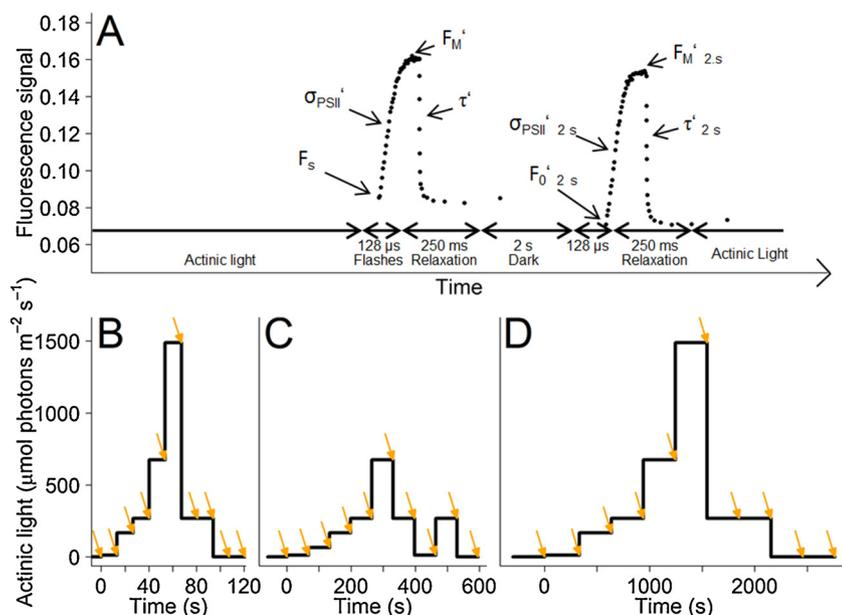
**Fig. 1.** Fluorescence measurement and light treatment protocols. 1A, FRRf protocol applied at each light step, with an induction/relaxation curve applied on top of actinic light, and then again after 2.5 s of darkness to allow re-opening of PSII. 1B, 10 s, 1C, 60 s and 1D, 300 s durations for light exposure periods in treatment protocols. Arrows indicate timing of applications of the FRRf measures during the light treatment protocols.
